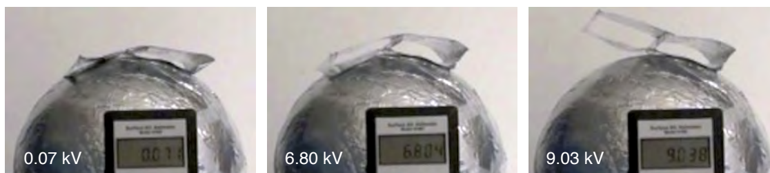
Figure 2.5: Electrostatic Inflation of a test sandwich structure, from 0 kV to 9 kV
