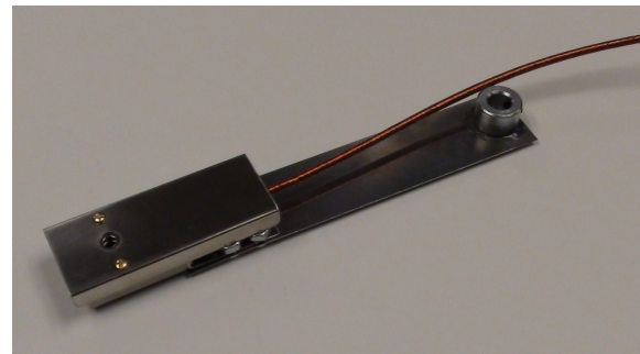
(b) Mounted faraday with collar for attachment to vacuum feedthrough
