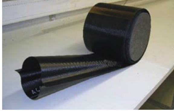
Figure 3.6: DLR's cylindrical inflatable boom (deploytech.eu)
