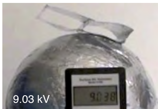
Figure 3.9: Electrostatically inflated 2-membrane sandwich structure
