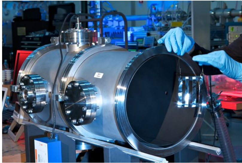
Figure 2.8: Vacuum chamber used for electrostatic inflation demonstrations and experiments
