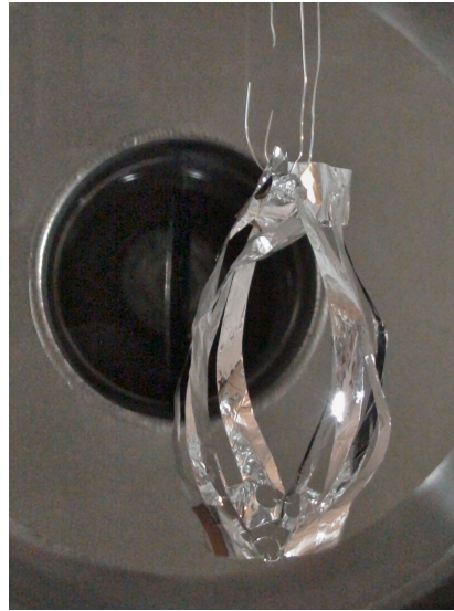
Figure 2.9: Electrostatic Inflation of membrane structure within the vacuum environment
